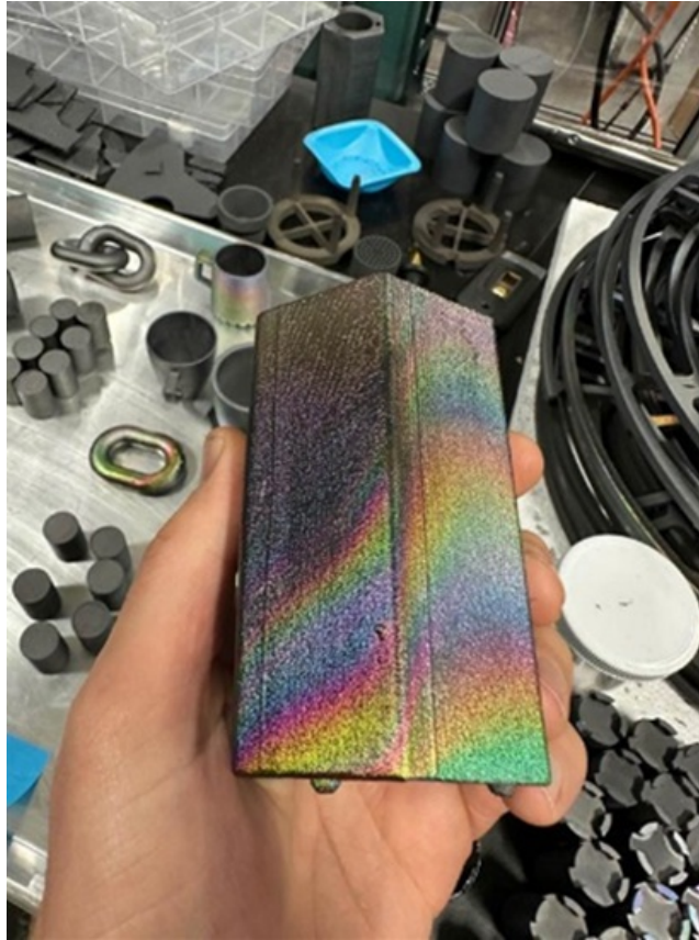
Figure 3. Additively manufactured, chemical vapor infiltrated SiC Pylon fuel element with prototypic size and shape and material. Filled with SiC surrogate powder.
