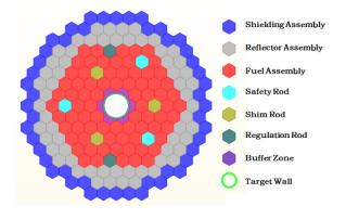
FIG.18. Scheme of CLEAR-I core
