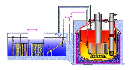
FIG. 7. Schematic representation of FBR-1 & 2
