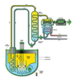
FIG. 1. Schematic representation of SFR
