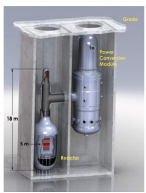
FIG. 30. EM2 reactor and gas turbine
