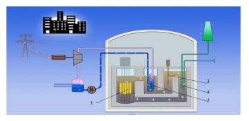
FIG. 23. BREST-OD-300 coolant circulation circuit
