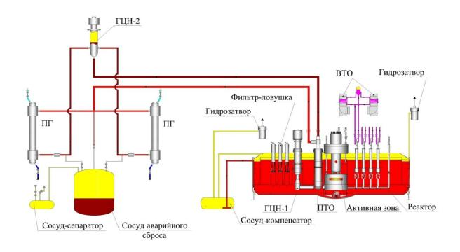
FIG. 11. Schematic view of BN-1200
