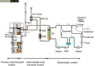
FIG. 8. Simplified plant schematic.
