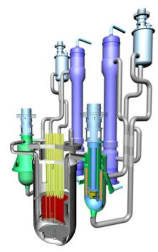
FIG. 9. Schematic Representation of JSFR.
