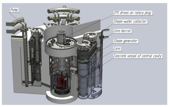
FIG. 22. Schematic representation of BREST-OD-300
