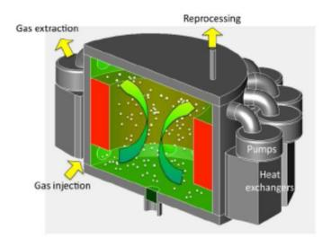
FIG. 4. Schematic representation of MSFR
