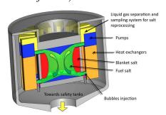
FIG. 32. Schematic MSFR design showing the fluoride-based fuel salt (green) and the fertile blanket salt (red).
