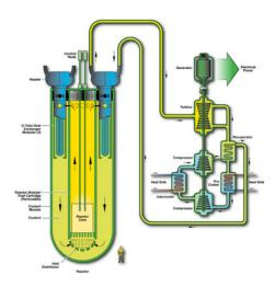
FIG. 2 Schematic representation of HLMC reactor
