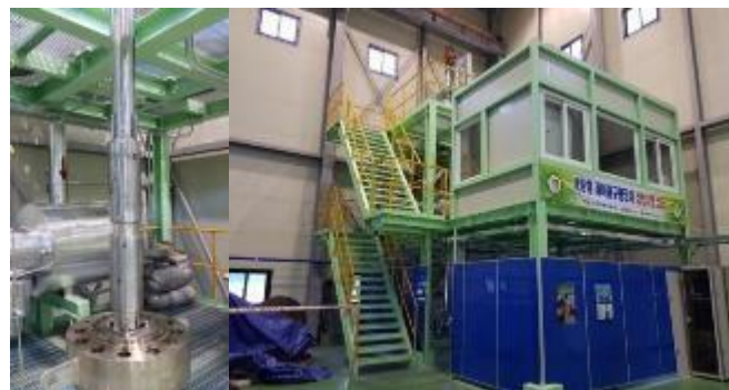
In-Vessel CRDM Demonstration Test Facility
