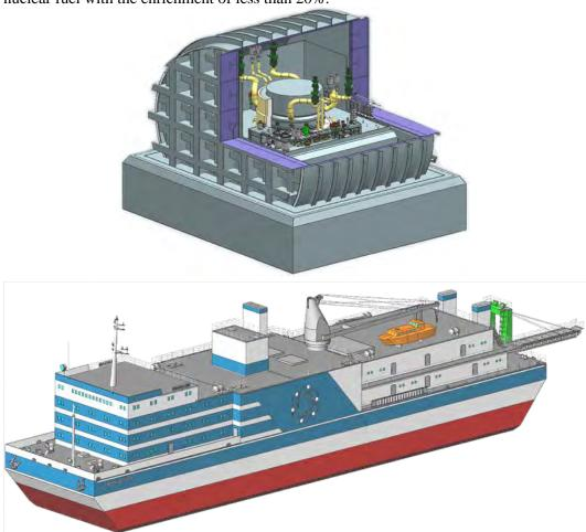
FPU includes reactor, steam-turbine, part of electric power system and control systems. The RPV operates under conditions of 16.2 MPa in the reactor pressure vessel. The steam generators located inside the RPV generate 295°C steam at 3.83 MPa flowing at 55 t/h. The RPV head is located under biological shielding and the control rod drive mechanism is located above the shield outside the vessel.
