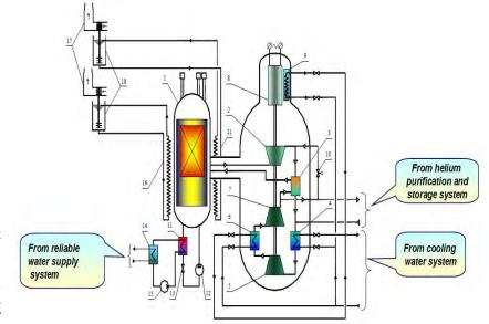
MHR gas turbine power conversion system has been made possible by utilizing large, active magnetic bearings, compact, highly effective gas to gas heat exchangers and high strength, high temperature steel alloy vessels.
