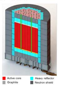
EM<sup>2</sup> core arrangement composed of fuel and reflector.
