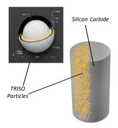
Fully Ceramic Micro-encapsulated (FCM<sup>TM</sup>) fuel
