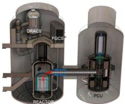
EM<sup>2</sup> primary heat transport system enclosed in two-chamber sealed containment
