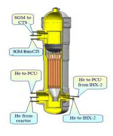
High Temperature Heat Exchanger Section
