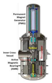
Power conversion unit and generator cutaway
