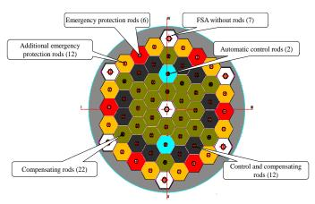
also be used to improve safety and fuel cycle characteristics. The SVBR-100 reactor pursues resistance to nuclear fissile material proliferation by using uranium with enrichment below 20% while using uranium oxide fuel in the initial core. The reactor is designed to operate for eight years without core refuelling.
