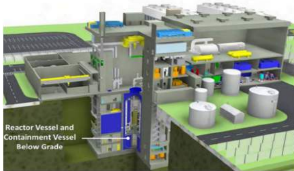
Below-grade location of Westinghouse SMR reactor and containment vessels
