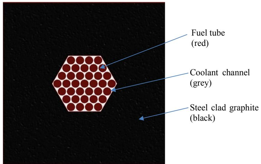
Figure 2: Section through fuel assembly showing the graphite, fuel tubes and coolant flow channel (Reproduced courtesy of Moltex)
