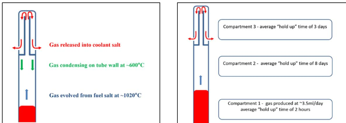
*Figures 3: Venting mechanism at the top of each fuel tube causes gaseous fission products to condense on the walls ensuring a hold up time before it is released to the coolant salt beyond the tube (Reproduced courtesy of Moltex)*
