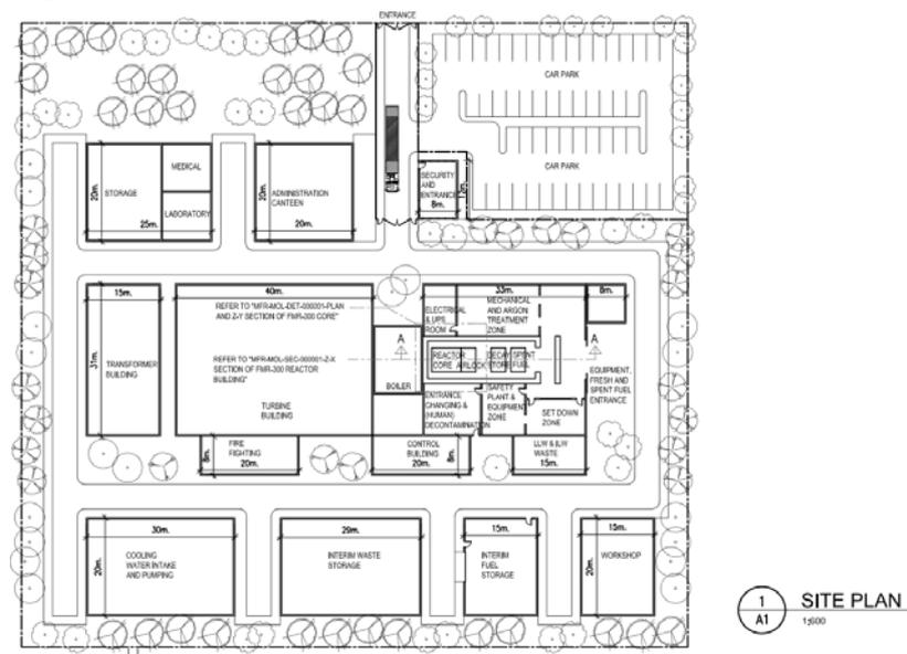
Figure 4: Illustrative site layout for a 300MWe plant (Reproduced courtesy of Moltex)
