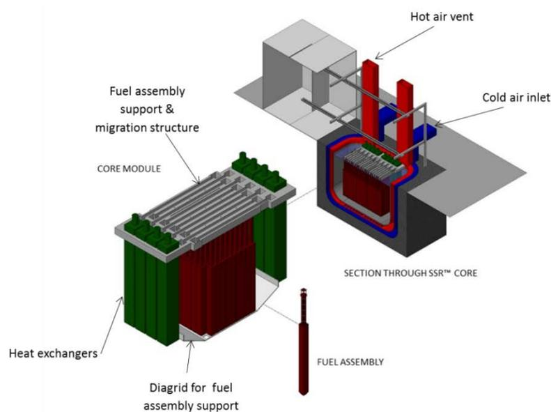
*Figure 1: Isometric view of core module and section through reactor (Reproduced courtesy of Moltex)*
