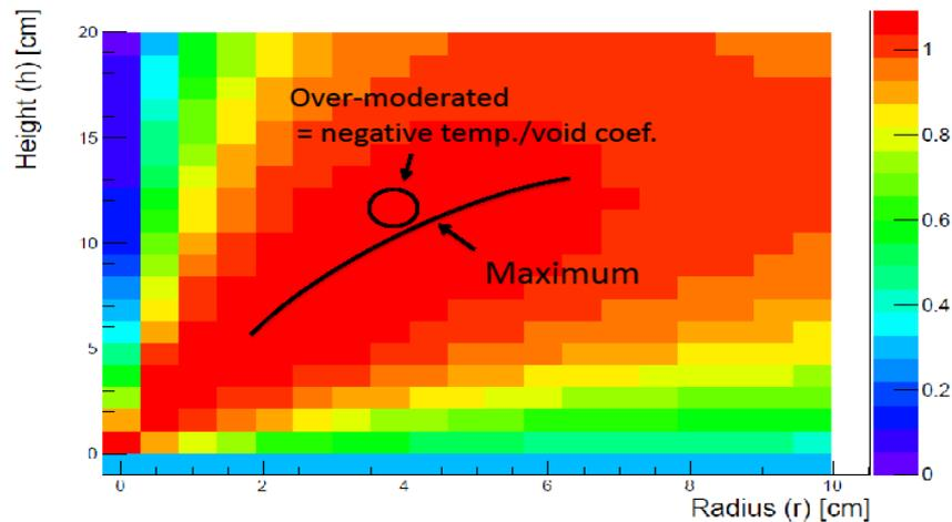
*Figure 2: Optimal configuration principle and safety through physics – illustrated through a core geometry optimization of  $k_{eff}$  (Reproduced courtesy of Seaborg Technologies).*
