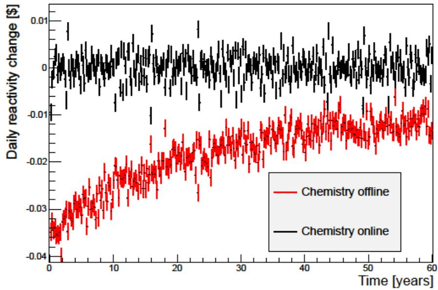
*Figure 4: Simulation of reactivity control using the chemical system. New spent fuel is added while fission products are continuously extracted, handled and vitrified.
