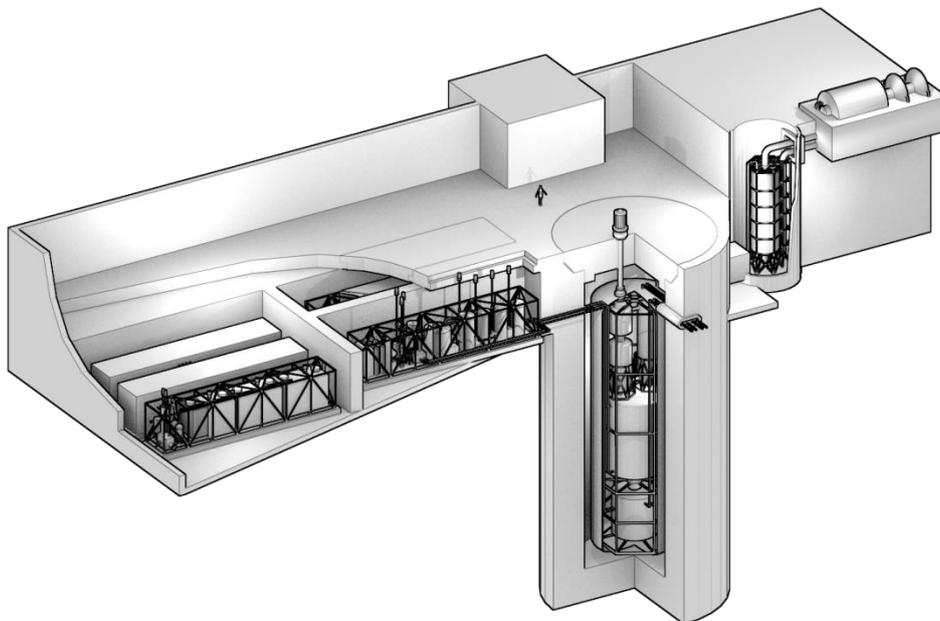
*Figure 1: View of the liquid-fluoride thorium reactor (LFTR) plant design
