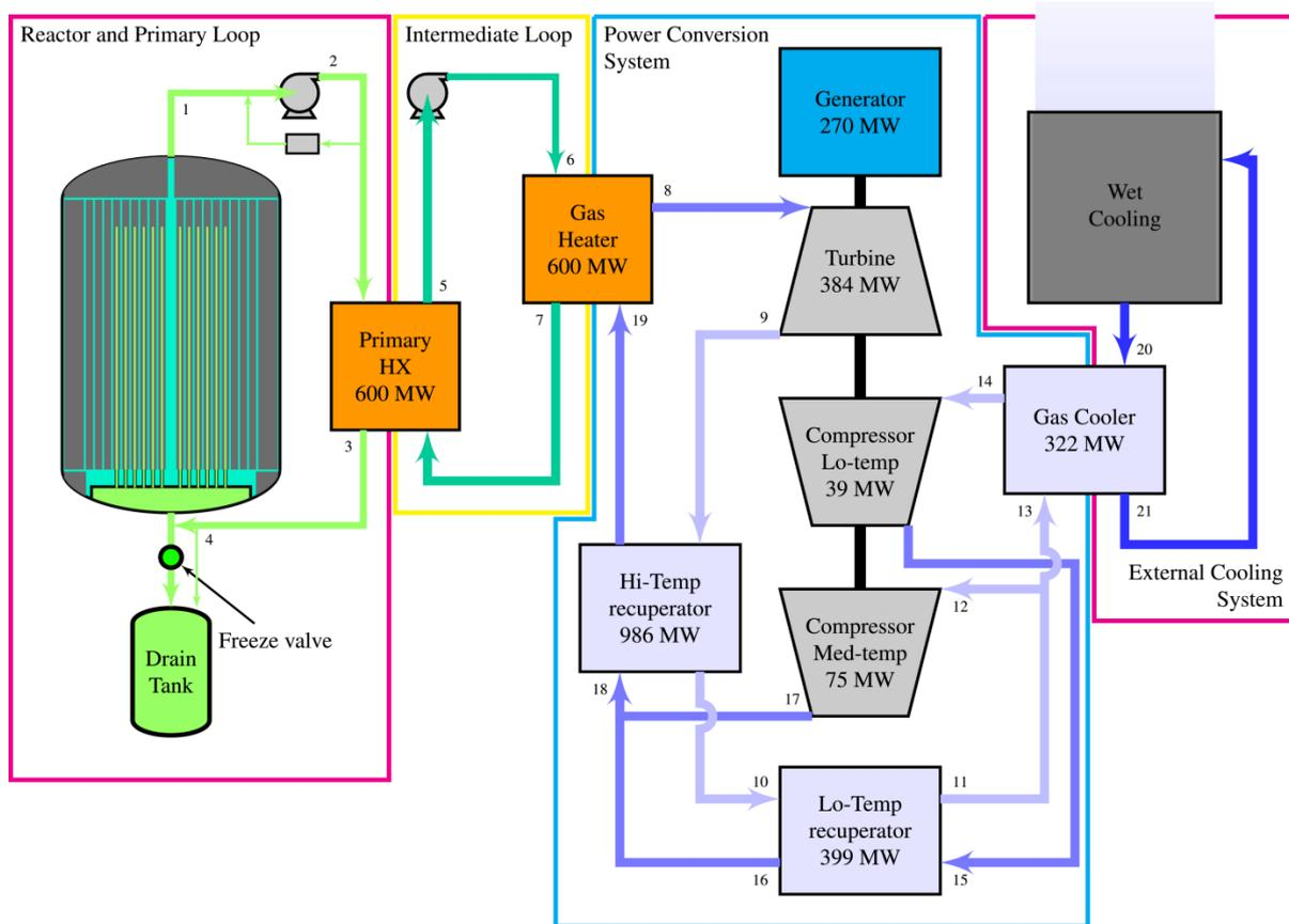
Figure 2: Reactor and primary loop, intermediate loop, power conversion system, and external cooling system simplified flow diagram (Reproduced courtesy of Fluide Energy)
