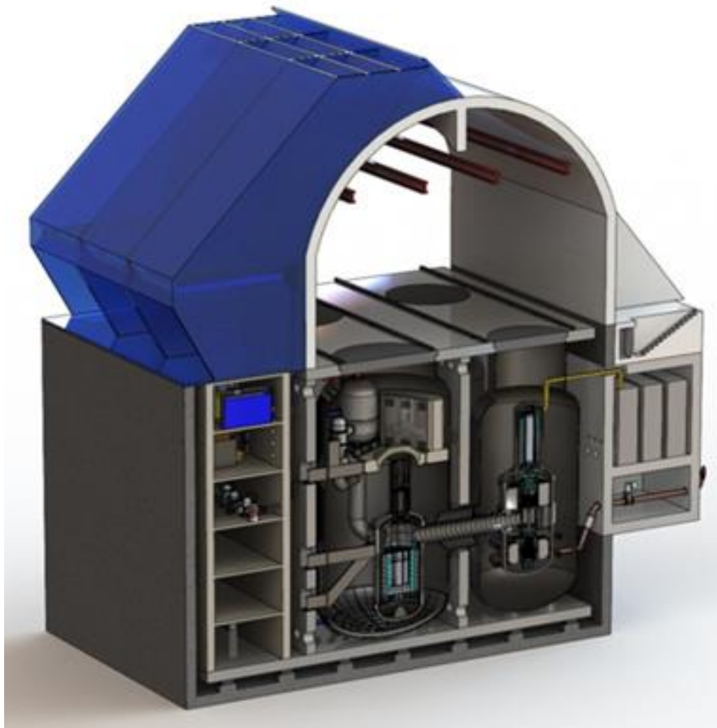
Fig. 1. Elevation view of EM 2 modular building element employing two modules on a single seismically isolated platform
