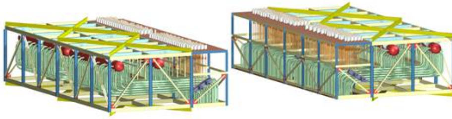
Figure 2-6 ACR-1000 Headers/Upper Feeders Modules
